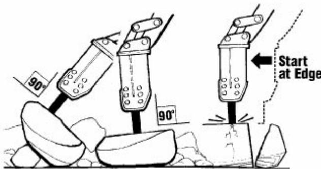
Damage can occur if the breaker is used for prying, picking or lifting.
